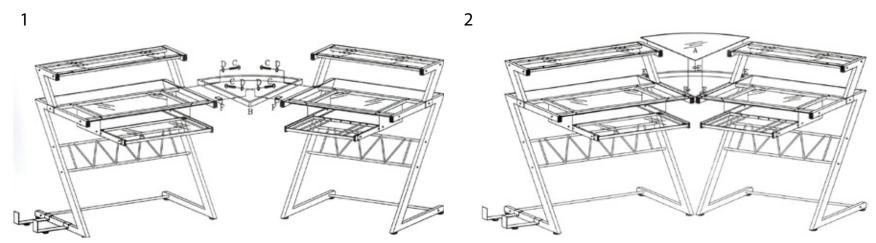
During assembly, hand tighten screws only. When all screws are in place, then tighten completely.
