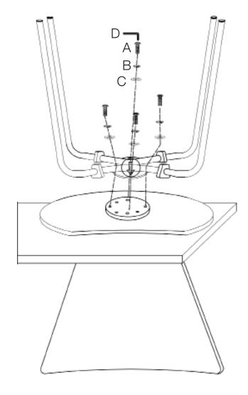
During assembly, hand tighten screws only. When all screws are in place, then tighten completely.
