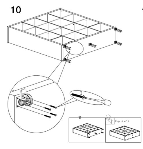
Install the casters as shown below and apply brakes on the casters when the shelf is at the desired location.
