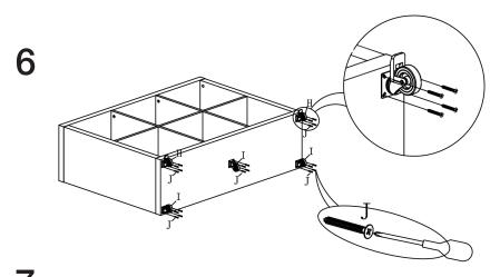
Install the casters as shown below and apply brakes on the casters when the shelf is at the desired location.
