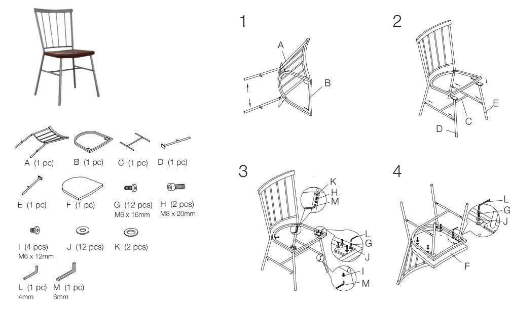
During assembly, hand tighten screw only. When the screw is in place, tighten completely.
