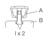
During assembly, hand tighten screws only. When the screws are in place, tighten completely.
