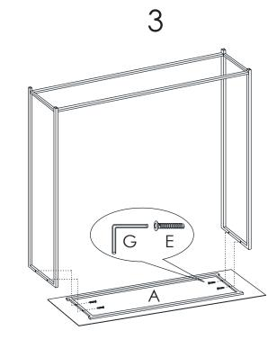
During assembly, hand tighten screws only. When the screws are in place, tighten completely.
