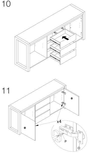
During assembly, hand tighten screws only. When the screws are in place, tighten completely. Assembly Instructions MANON Sideboard (Page 5 of 5 )
