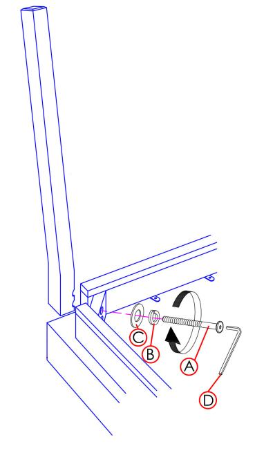
During assembly, hand tighten screw only. When the screw is in place, tighten completely.
