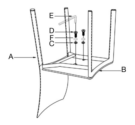
During assembly, hand tighten screws only. When all screws are in place, then tighten completely.
