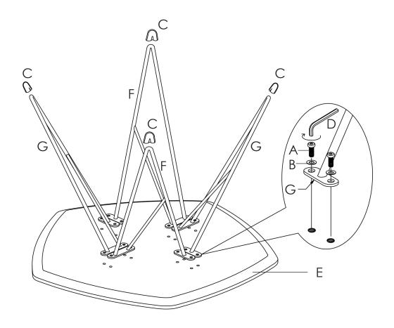
During assembly, hand tighten screws only. When the screws are in place, tighten completely.
