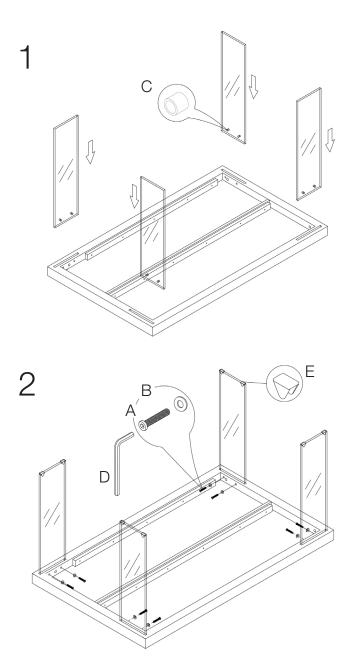
During assembly, hand tighten screws only. When the screws are in place, tighten completely.
