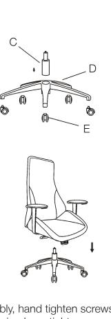
During assembly, hand tighten screws only. When the screws are in place, tighten completely.
