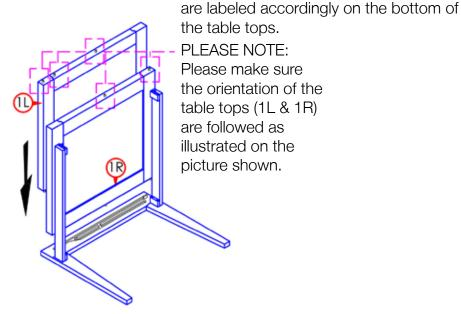
During assembly, hand tighten screw only. When the screw is in place, tighten completely.
