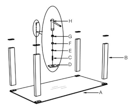
During assembly, hand tighten screws only. When all screws are in place, then tighten completely.
