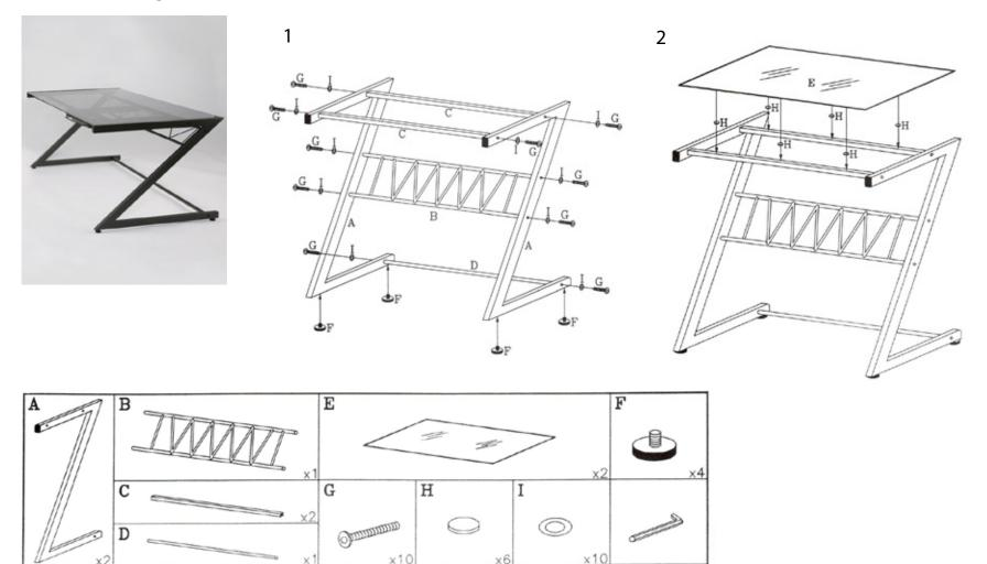
During assembly, hand tighten screws only. When all screws are in place, then tighten completely.
