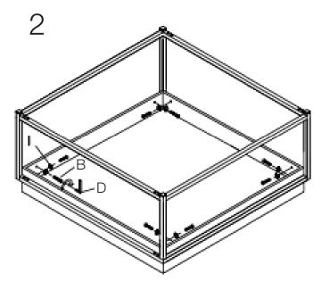
During assembly, hand tighten screws only. When all screws are in place, then tighten completely.
