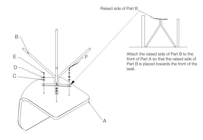
During assembly, hand tighten screws only. When all screws are in place, then tighten completely.
